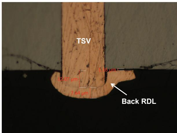
Fig.9 Cross section view after back RDL fabrication under the second process flow.
