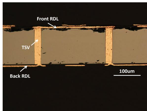
Fig.7 Cross section view after backside RDL fabrication under the first process flow.
