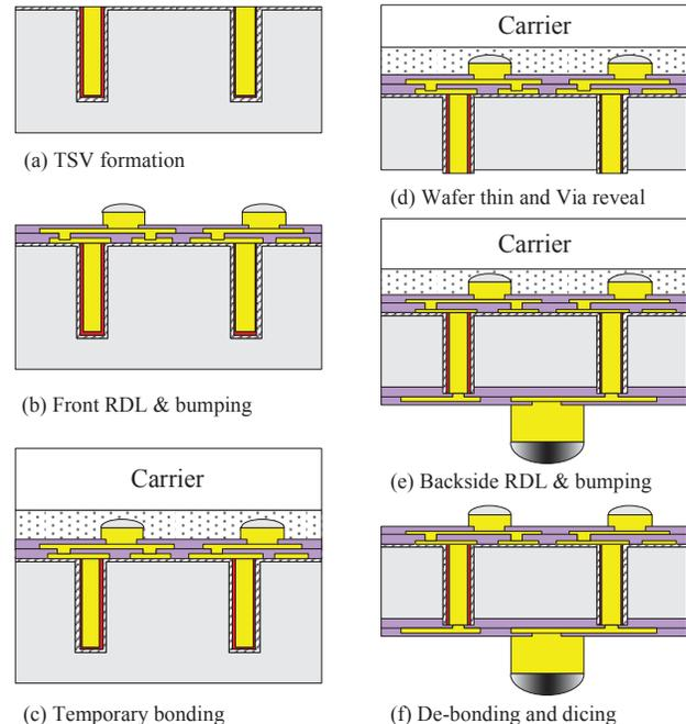
Fig. 1 Typical Process flow of TSV interposer.
