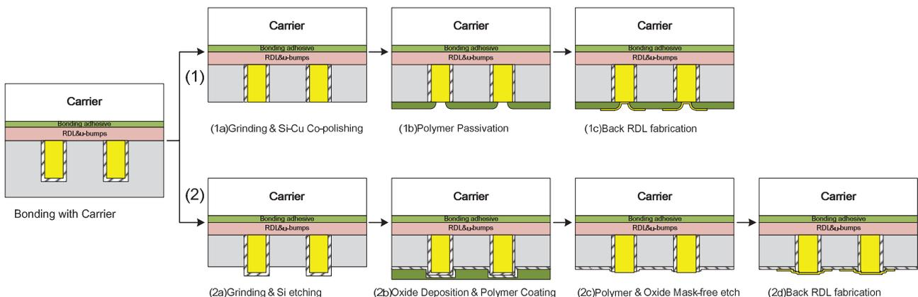
Fig.3 Proposed process flows for TSV Revealing
