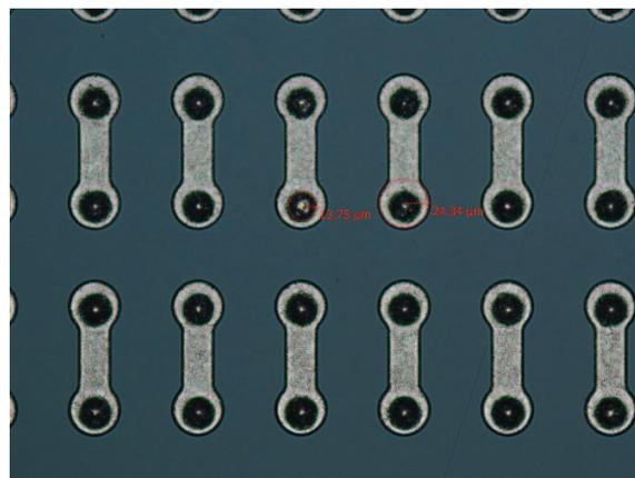
Fig.6 Surface microscope view after backside RDL fabrication under the first process flow.
