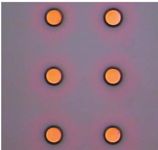
Fig.8 Surface microscope view after copper review under the second process flow.
