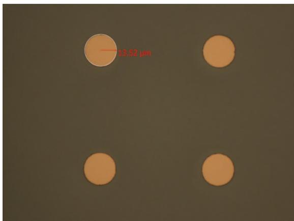
Fig.4 Optical Microscope view after copper reveal by Si-Cu co-polishing under the first process flow.
