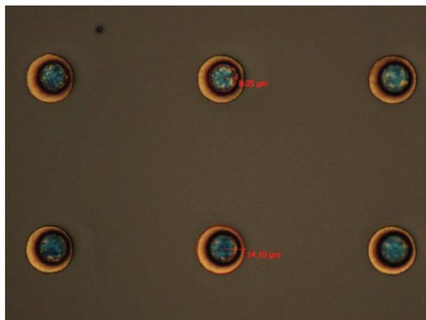
Fig.5 Optical Microscope view after backside passivation pattern opening under the first process flow.
