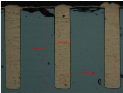
Fig.2 Cross section view of the TSVs filled with copper.
