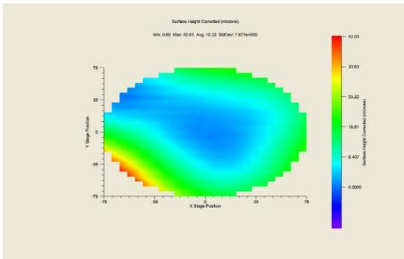
Fig.5 TTV of the coated bonding adhesives on a pillar bump wafer
