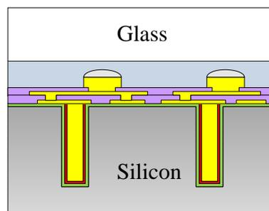
Fig.1 Typical temporary bonding structure for TSV interposers with RDL and micro-bumps
