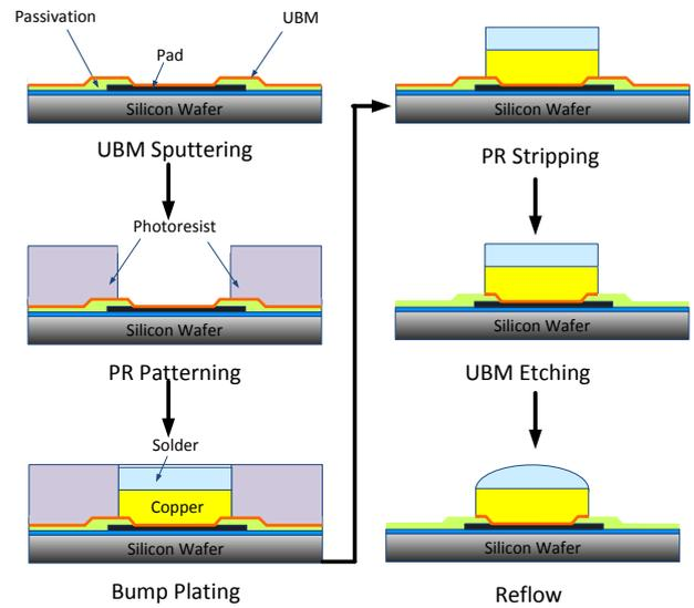
Fig.3 Process flow for fine pitch copper pillar bumps
