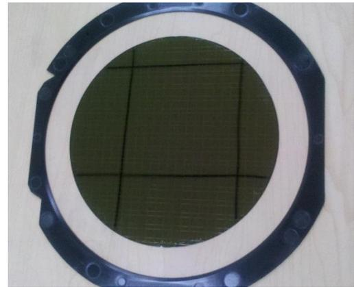
Fig.8 A successfully thermo-debonded wafer
