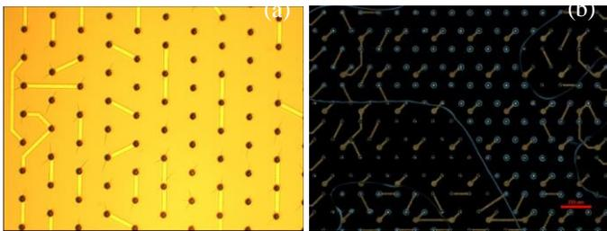
Fig.6 Optical pictures of (a) bubble free bonding and (b) bonding with visible bubbles
