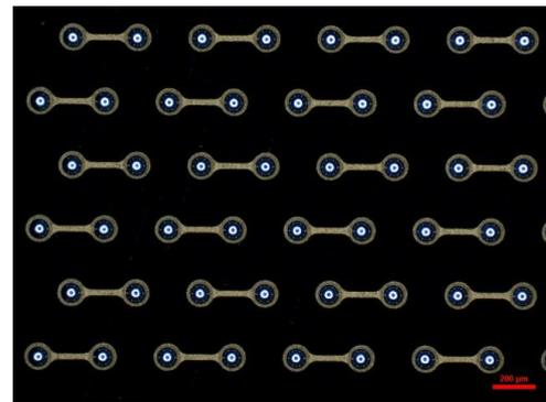
Fig.4 Optical picture of fabricated copper pillar bumps
