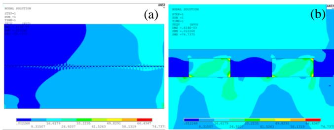
Fig.2 Overall stress distribution (a) and local stress distribution (b) for temporary bonded pairs
