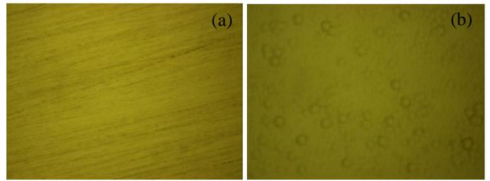
Fig.7 Wafer surface after (a) fine grinding and (b) dry etching
