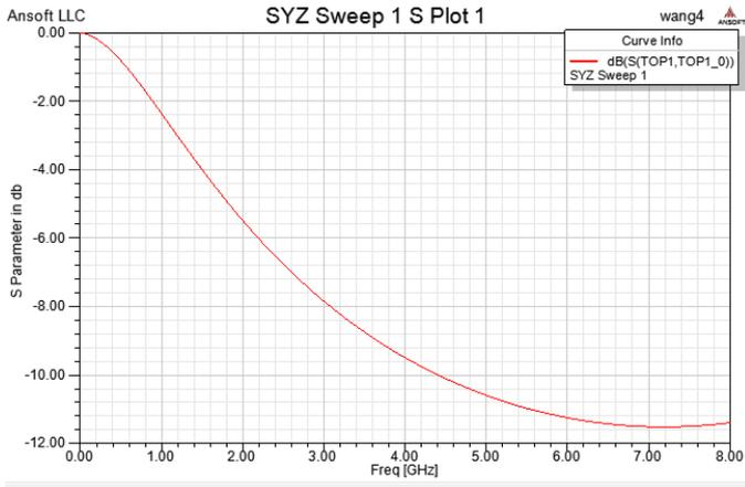
Fig1 show the isolation degree with frequency, when the surface structure size in the EBG have the 5x5 mm units metal microstrip
