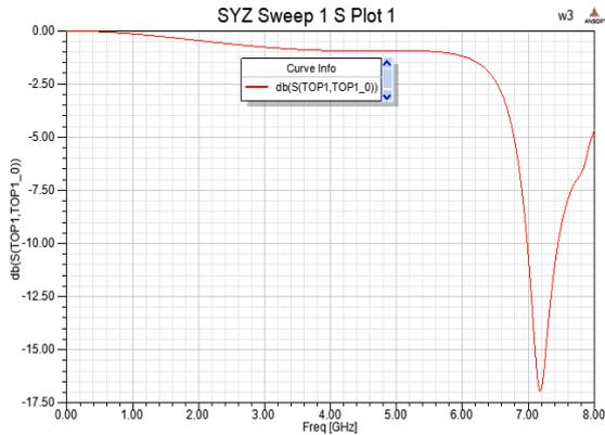
Fig5. |S<sub>21</sub>| of EBG structures with the value of a single capacitance buried inductance
