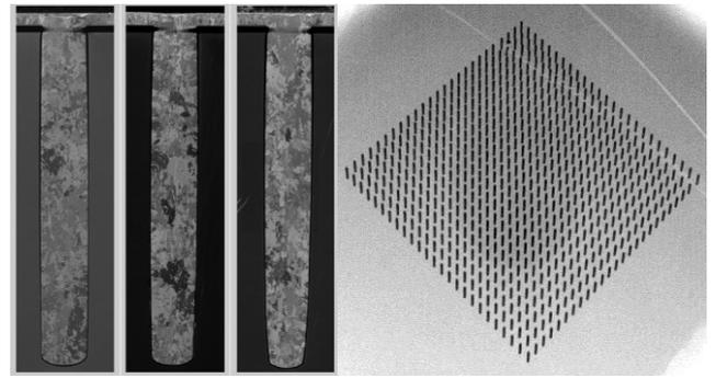
Figure 2 cross section and arrays of TSVs
