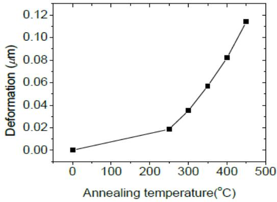
Figure 4 copper protrusion at different temperature
