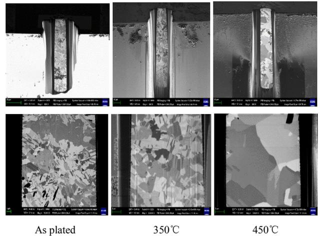
Figure 7 SEM of TSV without annealing at different test temperature
