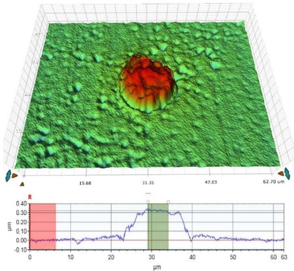
Figure 5 profile of TSV annealed at 300°C
