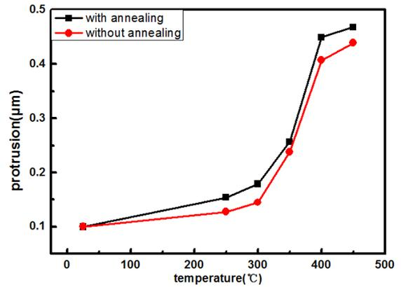
Figure 6 copper protrusion at different temperature by test
