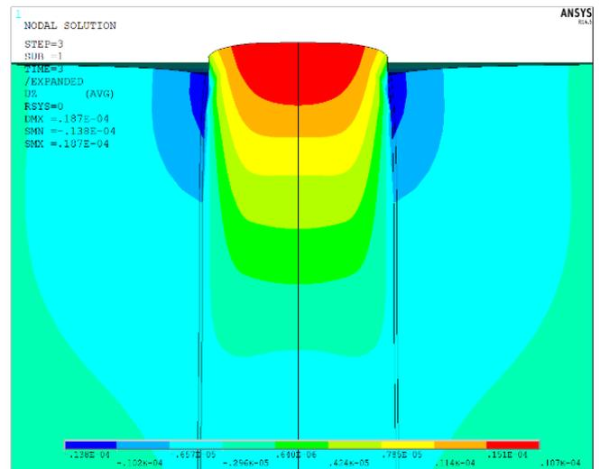
Figure 3 the simulation result of TSV protrusion
