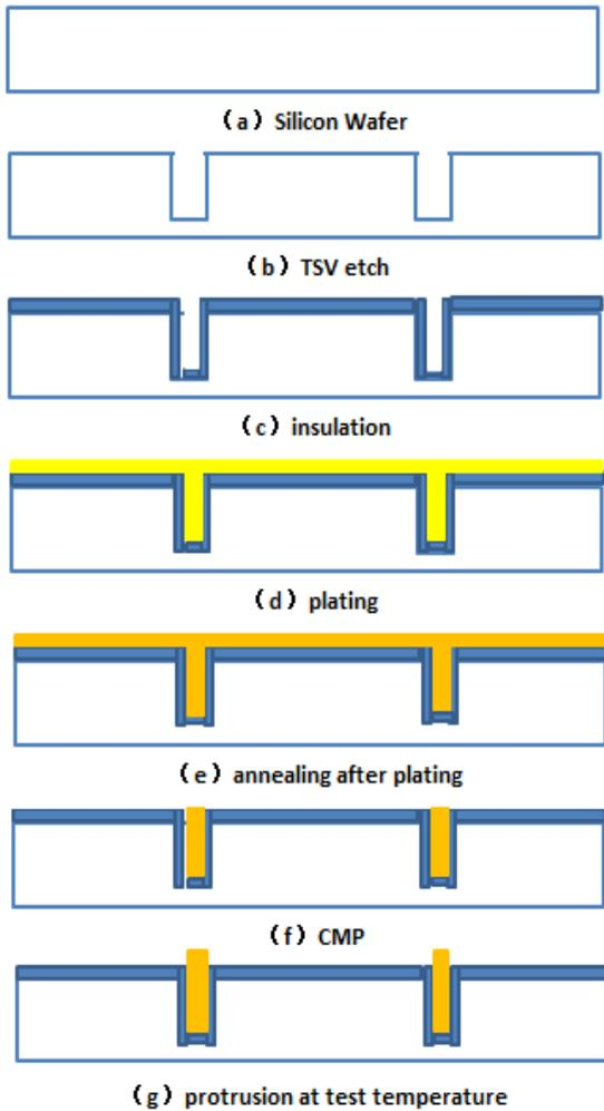
Figure 1 process flow of TSV fabrication
