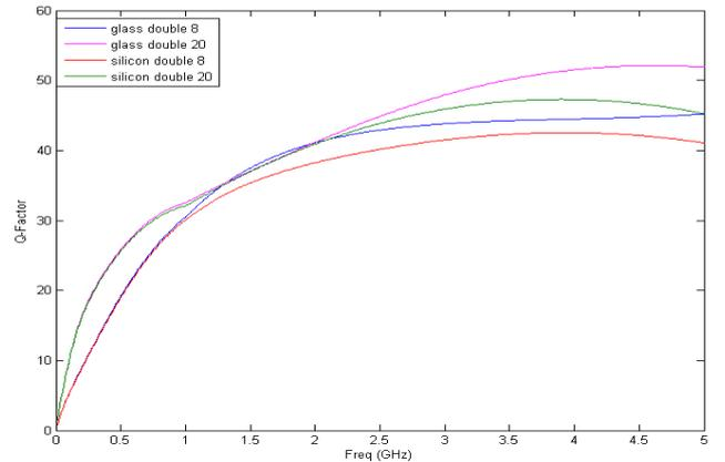
Fig. 5. Q-factor simulation result of the double-layer inductors
