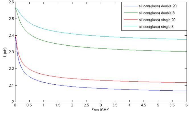
Fig. 4. Simulate  $L$  of inductors in silicon and glass substrates
