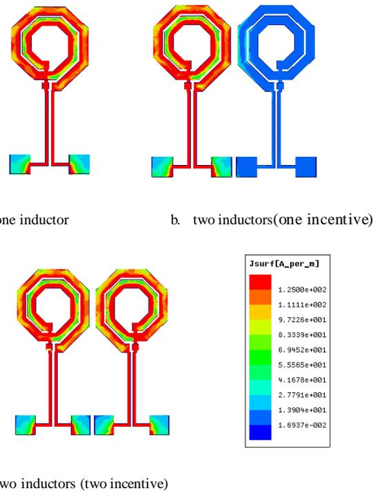
Fig. 10. Current density distribution of inductors
