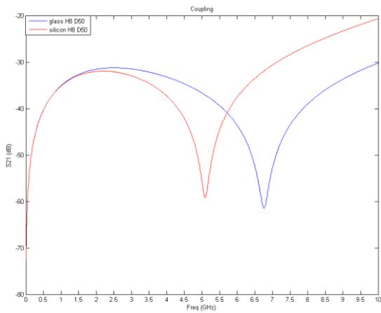
Fig. 7. Simulated response of two  $50\mu\text{m}$  apart inductors
