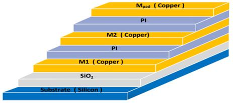
a. Inductors on silicon substrate
