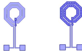
a. Single-layer inductor      b. Double-layer inductor
