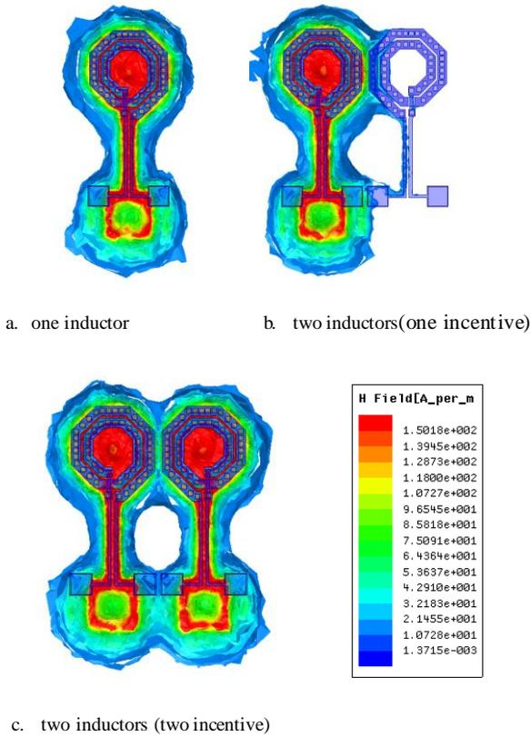
Fig. 11. Magnetic field distribution of inductors
