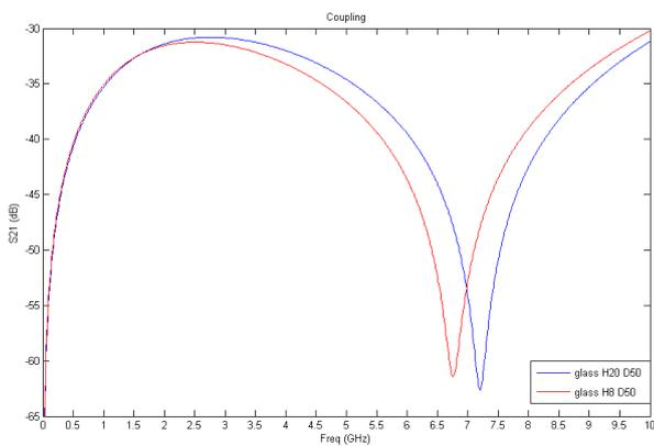
Fig. 8. Simulated response of two  $50\mu\text{m}$  apart inductors in glass substrate
