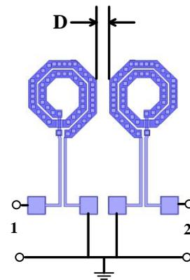
Fig. 6. Model for studying coupling
