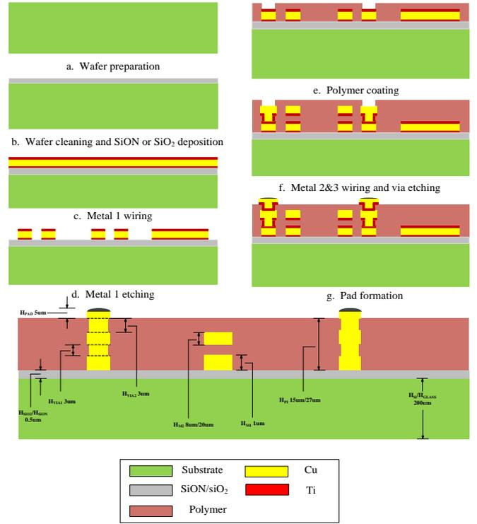
Fig. 2. Process flow for multilevel metal layers fabrication on glass and silicon wafer
