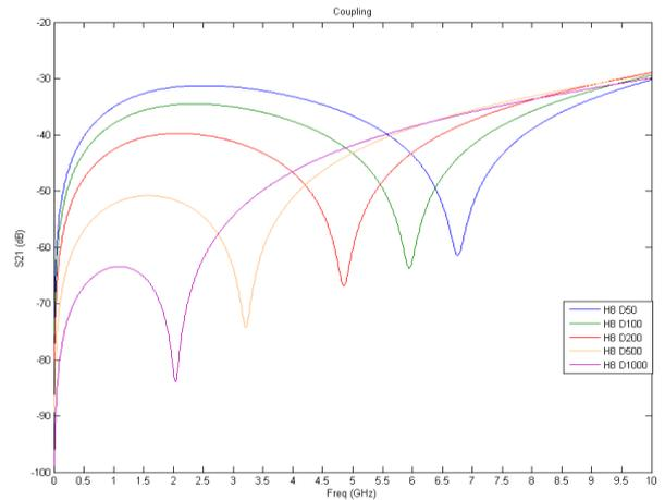
Fig. 9. Simulated response of two inductors in glass substrate
