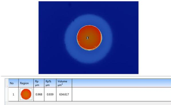
(b) Height and volume results measured by the analyzing software of the WLI
