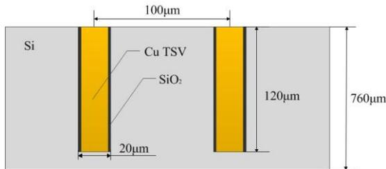
Fig.1 Schematic drawing of the TSV interposer
