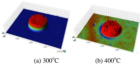
Fig. 5 Cu-TSV morphology after anneal test with CMP first approach
