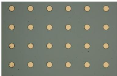
Fig. 2 Optical morphology of the polished TSV array
