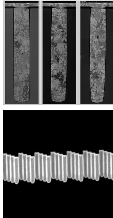
Fig. 3 Images of the cross section of the filled vias and their 3D X-ray image
