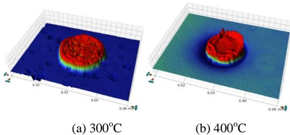
Fig. 6 Cu-TSV morphology after anneal test with anneal first approach
